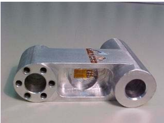
Figura 20 Prototype of torque sensor for the elbow joint.
