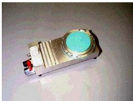
Figure 29 Underwater pressure compensated matrix tactile sensor (1999-2000).
