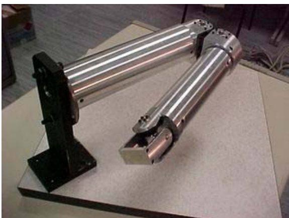
Figura 19 Prototype of the arm (4 d.o.f.). Elbow and wrist demonstrator
