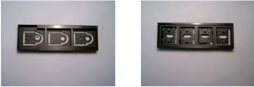
Figura 15 Machined parts. Adopting CAD-CAM tools allowed rapid prototyping of small series of parts.
