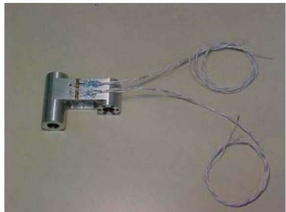
Figura 20 Prototype of torque sensor for the elbow joint.
