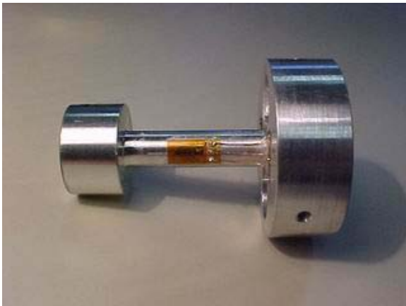
Figura 21 Prototype of joint torque sensor (and custom electronics)
