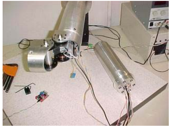
Figura 24 Preliminary integration and tests of the control nodes. Each node controls a single joint and nodes communicate through a CAN serial bus.
