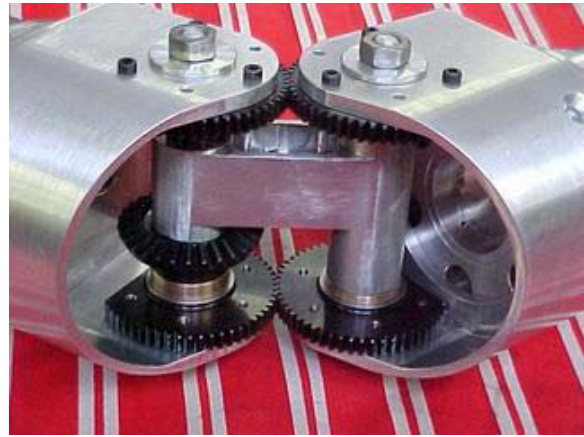
Figura 22 A particular elbow joint has been designed to allow complete flexion of the forearm.
