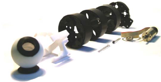
Figura 3 MACEYE - first prototype (july-september 2004). Tendon sensors not shown.
