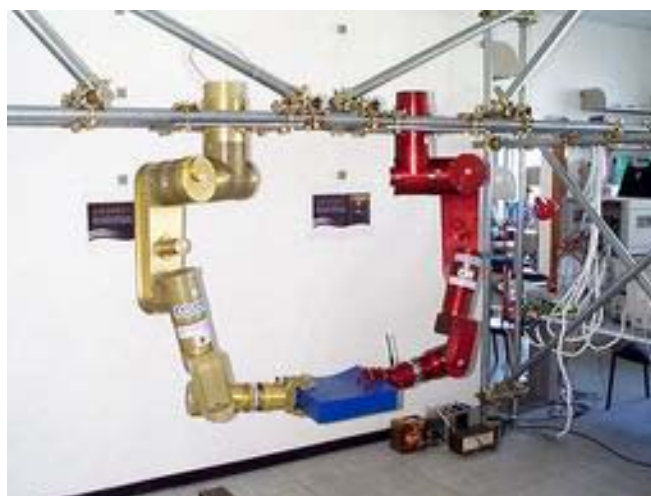
Figura 25 Dual arm underwater work-cell. Each arm has 7 degrees of freedom (1996-1999).
