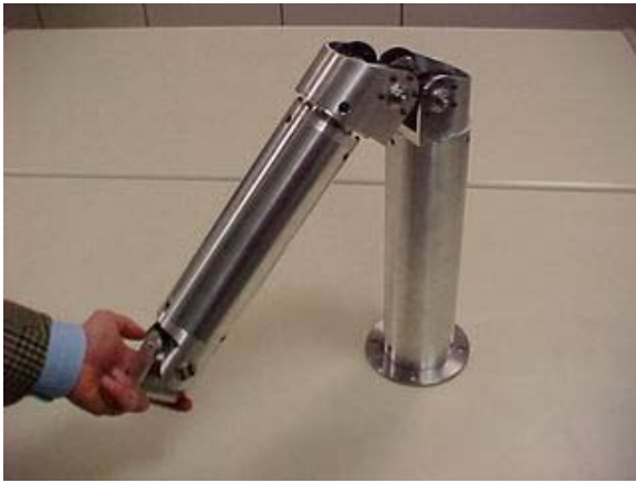
Figura 22 A particular elbow joint has been designed to allow complete flexion of the forearm.
