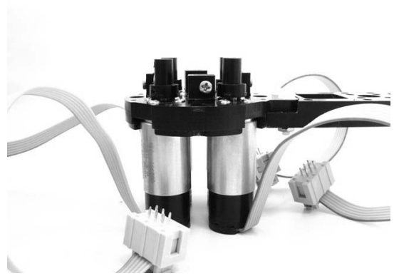
Fig. 12. Four DC motor actuate the tendons; pulleys (barely visible here) route the tendons towards the eye-ball.
